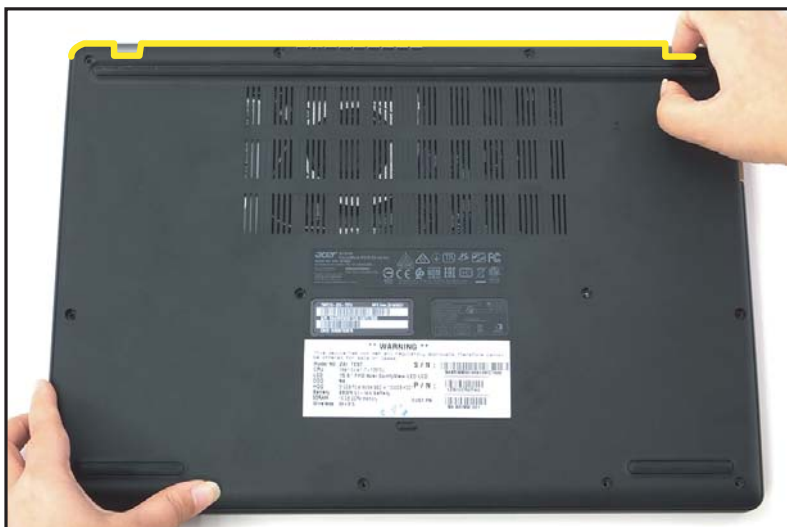
Figure 1-4. Base Cover Removal
