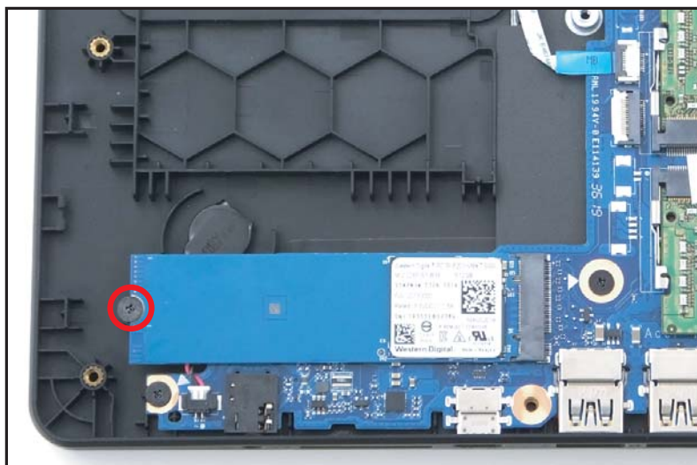
Figure 1-14. SSD Module Removal
