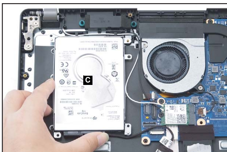
Figure 1-17. HDD Module Removal
