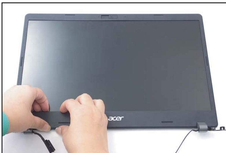
Figure 1-48. LCD Bezel Removal
