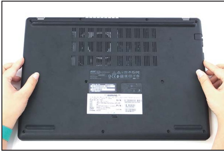
Figure 1-5. Base Cover Removal
