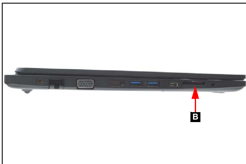
Figure 1-2. SD Card Removal
