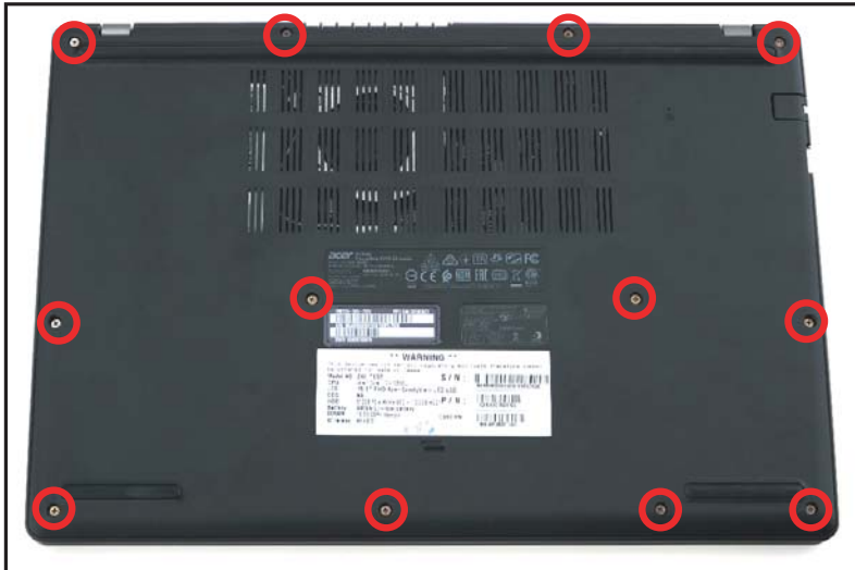
Figure 1-3. Base Cover Removal
