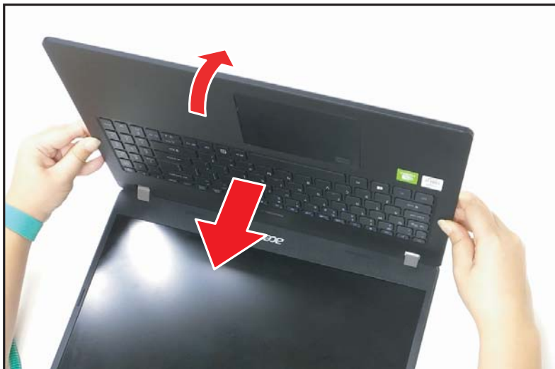
Figure 1-30. LCD Module Removal
