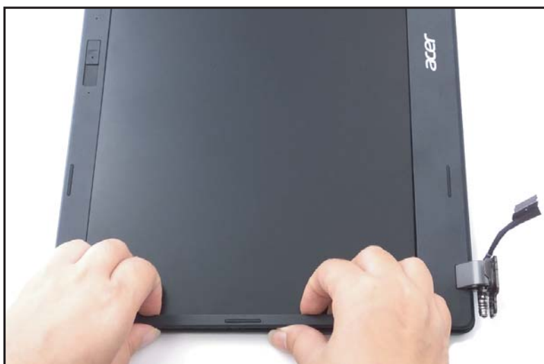
Figure 1-49. LCD Bezel Removal
