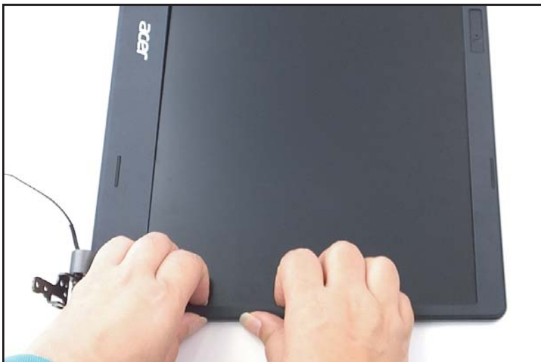
Figure 1-51. LCD Bezel Removal
