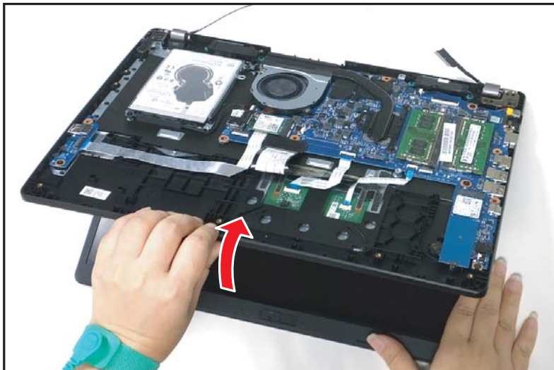
Figure 1-28. LCD Module Removal
