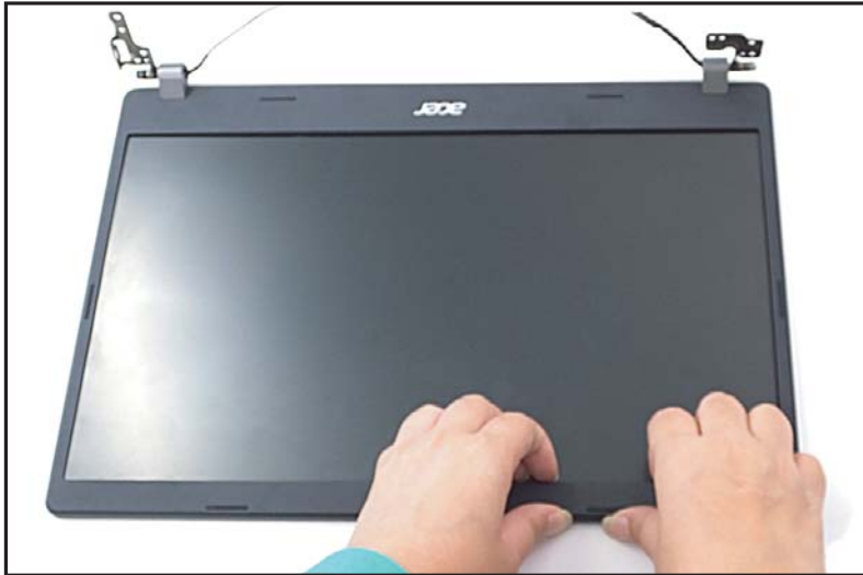
Figure 1-50. LCD Bezel Removal
