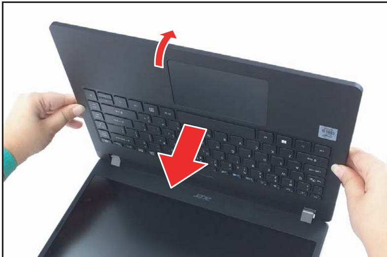
Figure 1-38. LCD Module Removal
